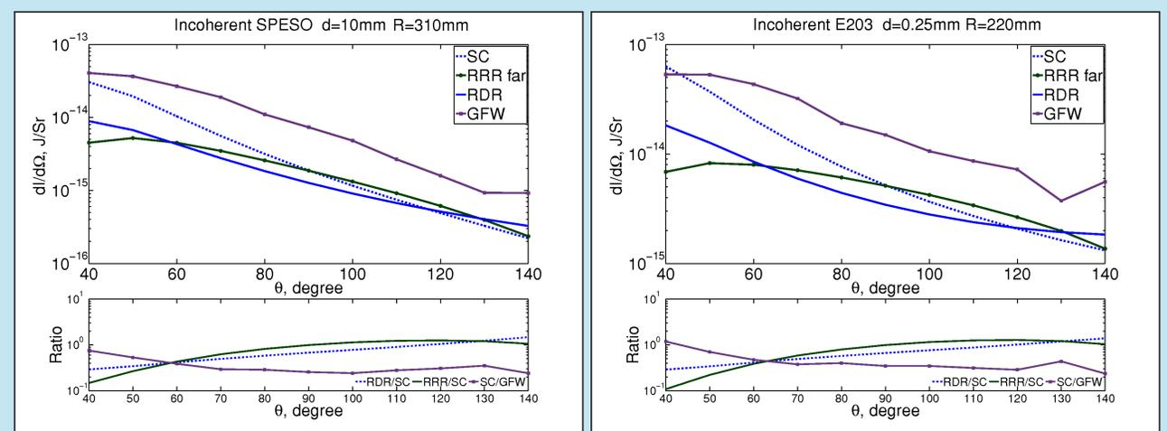
SPESO experiment parameters, d=10mm
